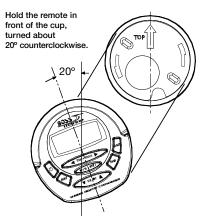
4. Insert the remote control fully into the cup so that the mounting hooks go through the slots in the back of the cup.
