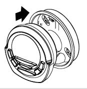
If you feel resistance when you insert the remote into the cup, pull the remote housing out and check that the cable has been pressed into the curved slot, as described in Step 2).
